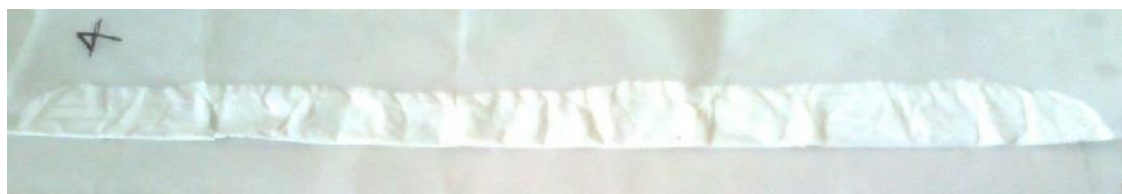
Fig 1 Determination of hard and sharp edged abrasive particles
