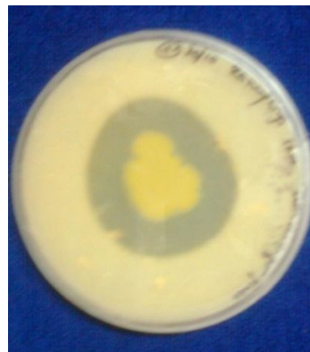
Figure 3.1 Zone of hydrolysis around the colony of K3 on skim milk agar plate.
