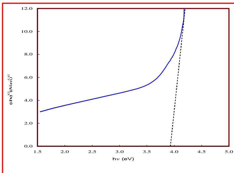
Fig. 2: Urbach plot for evaluating the optical band gap of NaF-Al<sub>2</sub>O<sub>3</sub>-B<sub>2</sub>O<sub>3</sub> glass system
