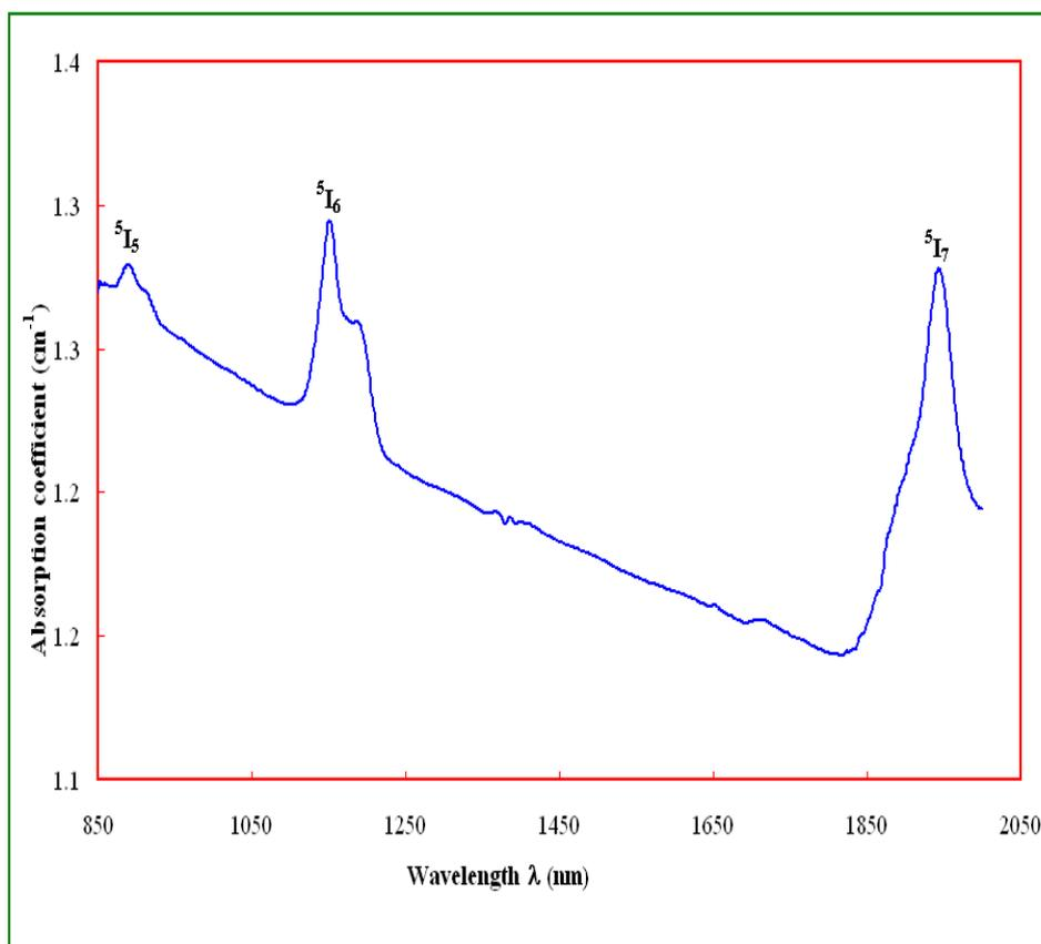
**Fig. 4:** Optical absorption spectrum of NaF-Al<sub>2</sub>O<sub>3</sub>-B<sub>2</sub>O<sub>3</sub> glass system doped with 1.0 mol % of Ho<sub>2</sub>O<sub>3</sub> recorded at room temperature (NIR region)
