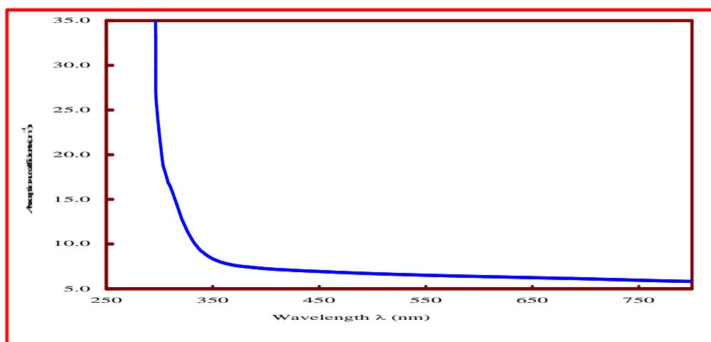
**Fig. 1: Optical absorption spectrum of NaF-Al<sub>2</sub>O<sub>3</sub>-B<sub>2</sub>O<sub>3</sub> glass system recorded at room temperature**
