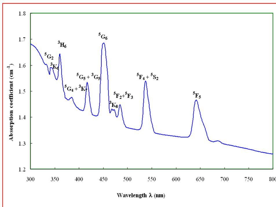
Fig. 3: Optical absorption spectrum of NaF-Al<sub>2</sub>O<sub>3</sub>-B<sub>2</sub>O<sub>3</sub> glass system doped with 1.0 mol % of Ho<sub>2</sub>O<sub>3</sub> recorded at room temperature
